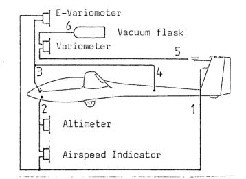
When connecting an electrical variometer (E.V.) additionally to the boom static ports (tube No. 4), a blowing circuit must be switched operative to avoid water entering system during water ballast discharge. Thus the electrical variometer is inoperative during water discharge. Important Note: Manual operation of blowing circuit during water discharge
