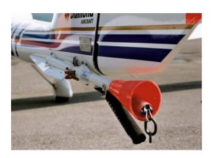
Integral tail support with rope pullout sensor, lop system for emergency release and hard points for mounting an optional standard bolt
