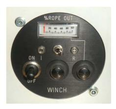
Indicator with an automatic system shut-down after retracting, including an integrated adjustable rope length indication
